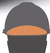
**2** Integral, perforated sweatband puts barrier between **HEAD** and **HEADBAND**
